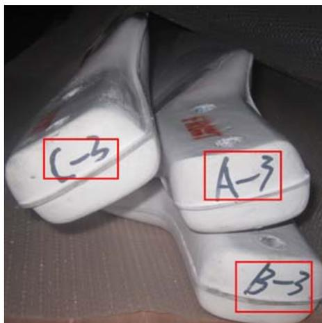
5.7 The blades should be kept horizontal on the ground when installing the hub;
