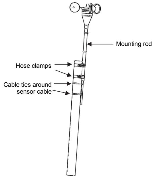
3. Tighten the hose clamps making sure the mounting rod remains vertical.
