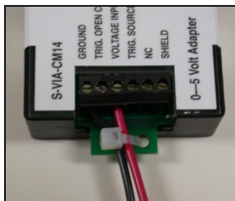
Figure 1: Cable strain relief
